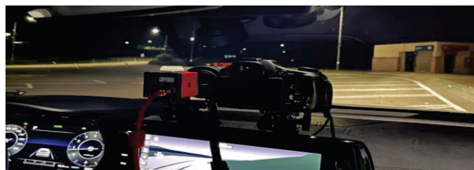
Fig. 1. Installation of a Camera Inside a Vehicle for a Survey
