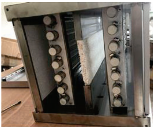
Fig.5 UVC lamp and ceramic photocatalyst mesh plate in microwave cavity
