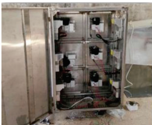
Fig. 6 Photocatalytic equipment combined with 6 sets of microwave cavities
