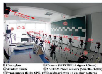
Fig 8. Test room setup for the validation study.
