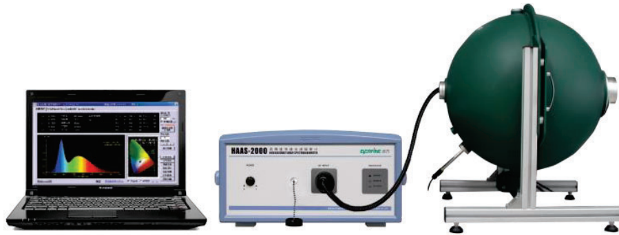
Figure 6. EVERFINE HAAS series high accuracy spectrometer
