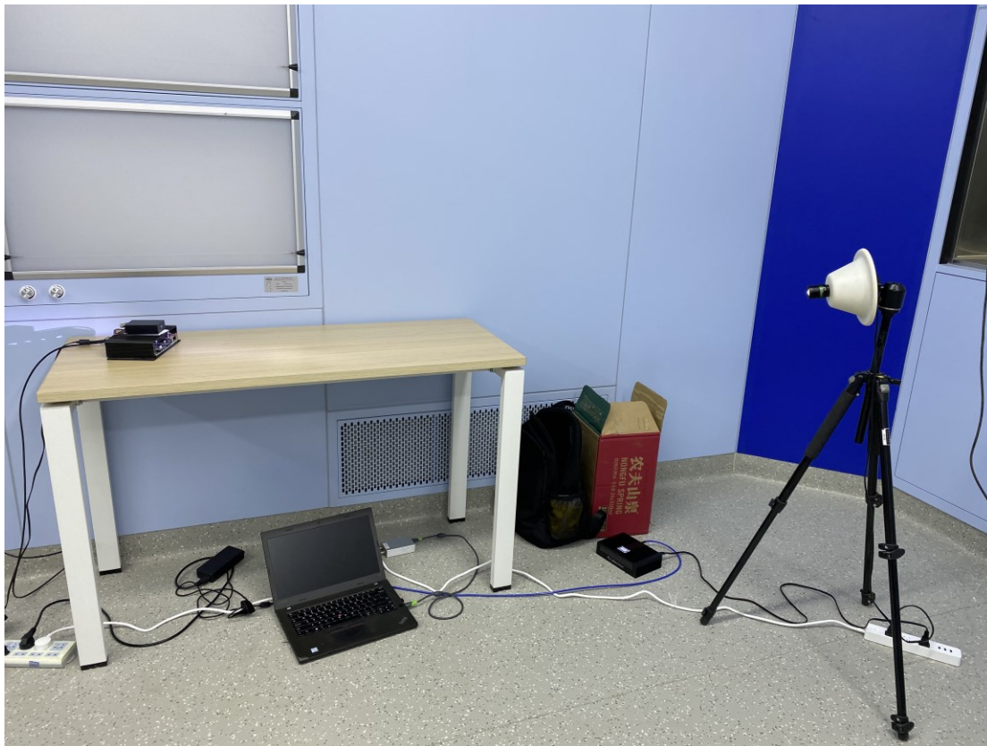
Fig2. VLC video transmission system used in the digital operation room
